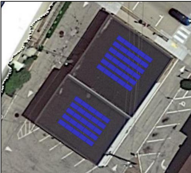
3. 22.6-kw DC fixed-tilt roof mounted array on the Police Station Location
