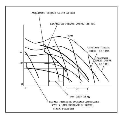
QT=FAN AIRFLOW-CFM-STANDARD AIR SP=FAN STATIC PRESSURE-IWC IWC=INCHES WATER COLUMN
