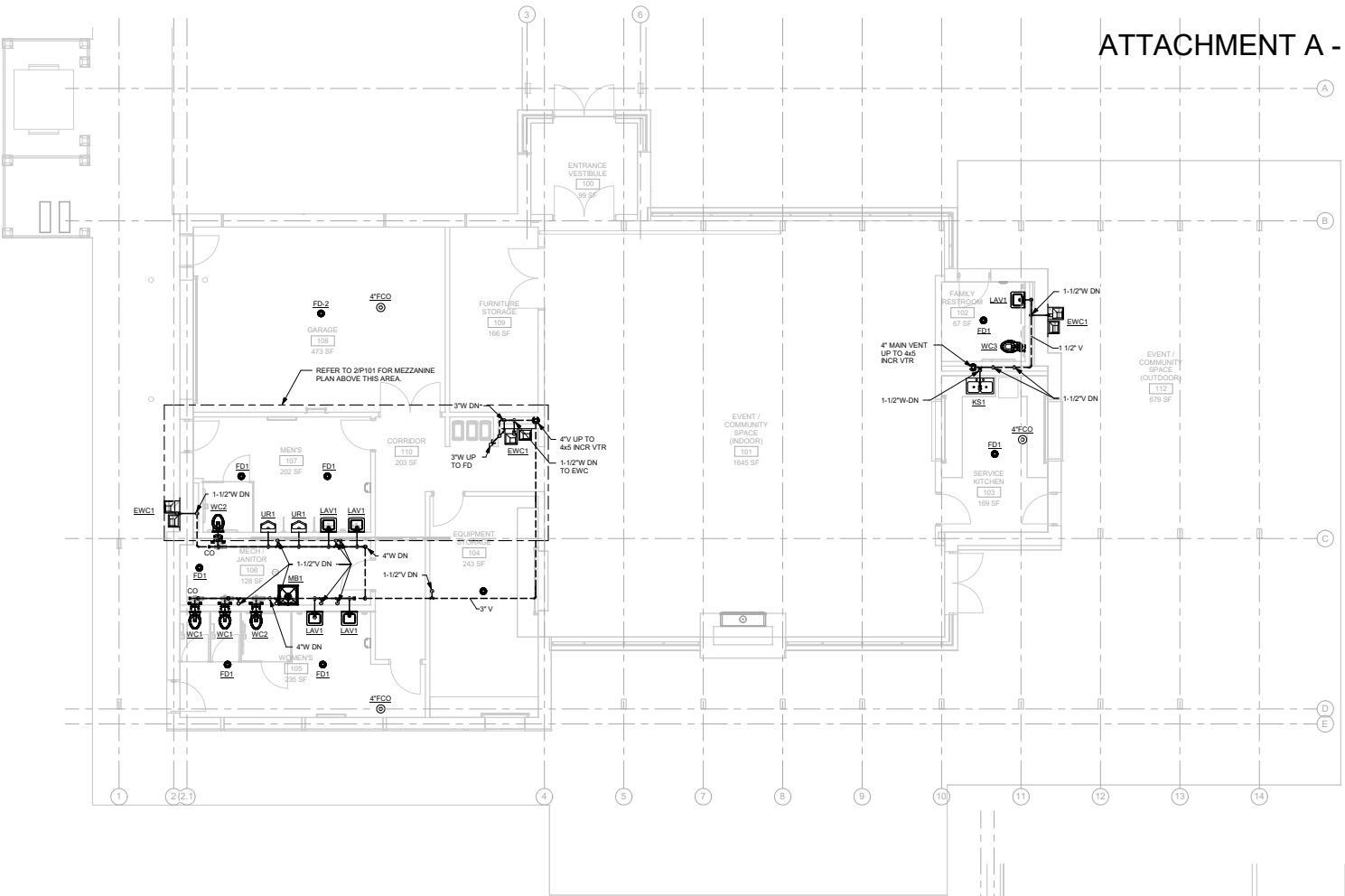
FIRST FLOOR PLUMBING PLAN - DWV 3/16" = 1'-0"
