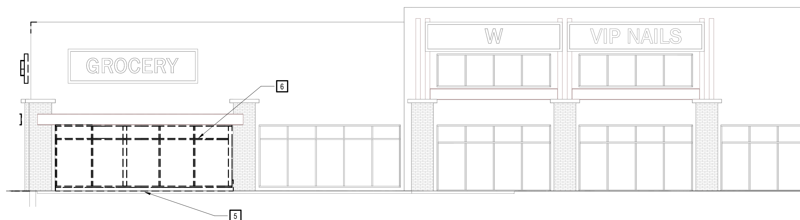
3 EXISTING GROCERY STORE DEMO ELEVATION - EAST SCALE: 1/8" = 1'-0"
